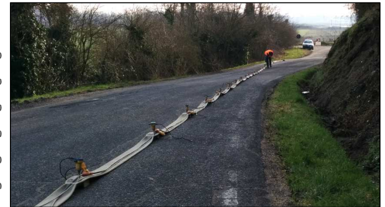
Figure 2 - Land Streamer with regular spaced geophones
